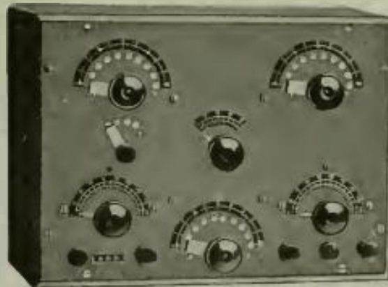
Regenerative Receiver, 200-2500 meters
